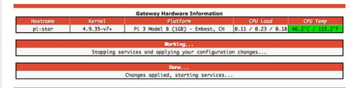
Clicking any of the Apply Changes buttons will apply all changes made in any of the sections, but it's a good idea to apply changes after working in each section. For example, if you have enabled various modes (DMR, D-STAR, etc.), the associated configuration section is displayed only after you apply your changes.
